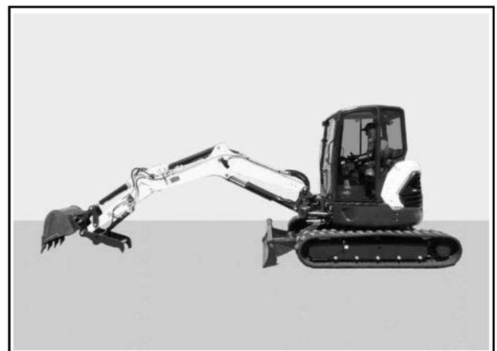
3. Position the excavator with the bucket fully rolled out and the arm fully extended [Figure 211].
