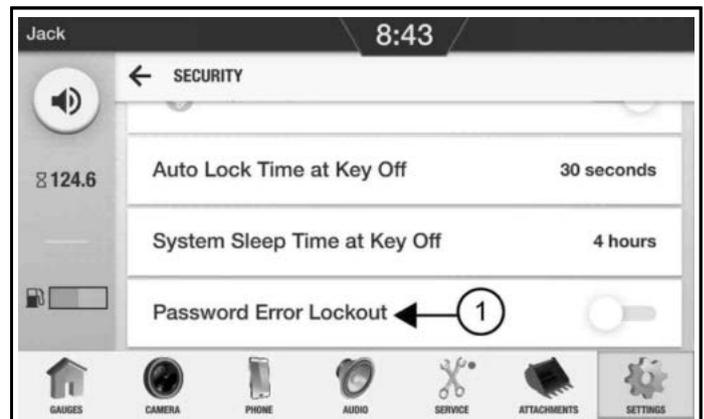
2. Select **[PASSWORD ERROR LOCKOUT]** (Item 1) [Figure 463] to turn on / off.
