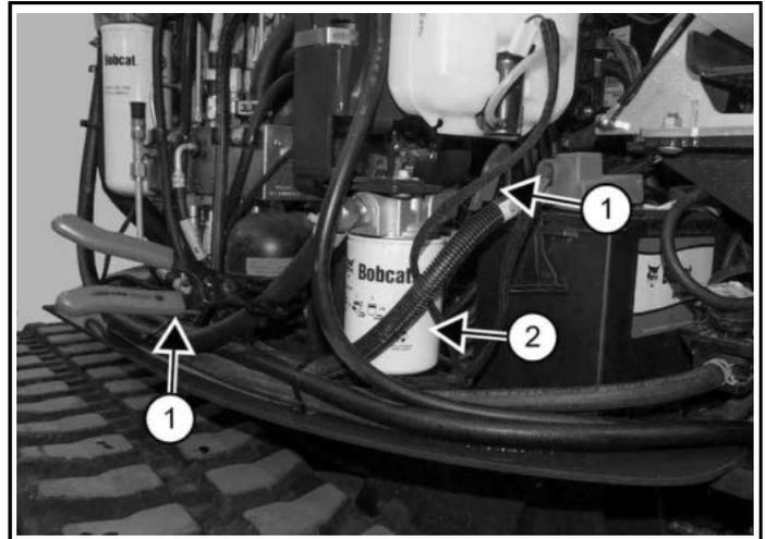
5. Install locking hose pliers (Item 1) [Figure 368] on the hoses running to the filter housing.
