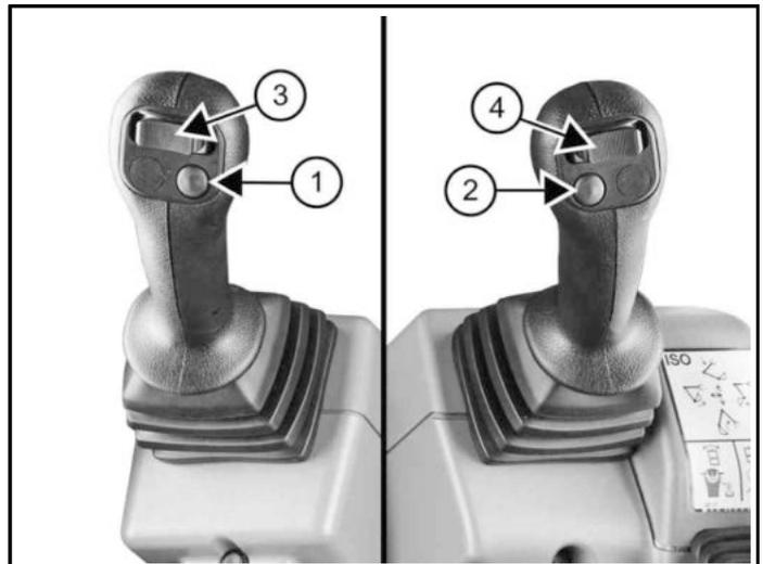
3. Press the joystick buttons to toggle to the desired joystick control configuration.
