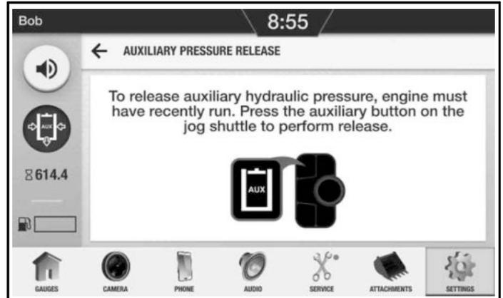
5. To release auxiliary pressure, press the AUX button on the jog shuttle as shown on the screen [Figure 444].
