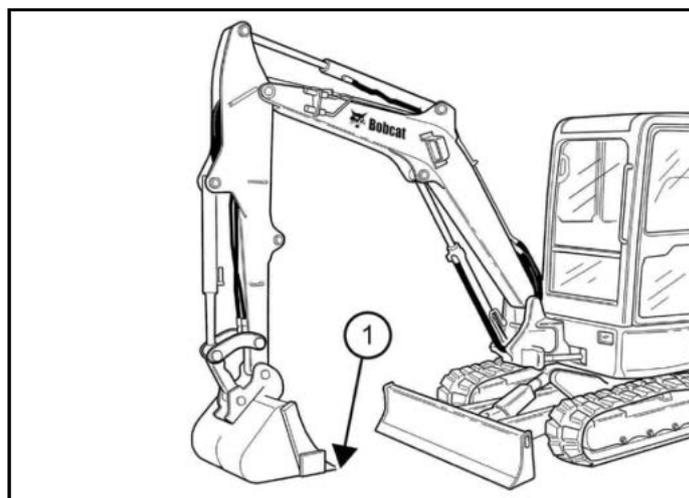
1. Set the bucket (Item 1) [Figure 288] on the ground surface where you are going to start the dig or on the surveyor mark to establish the starting ground position.
