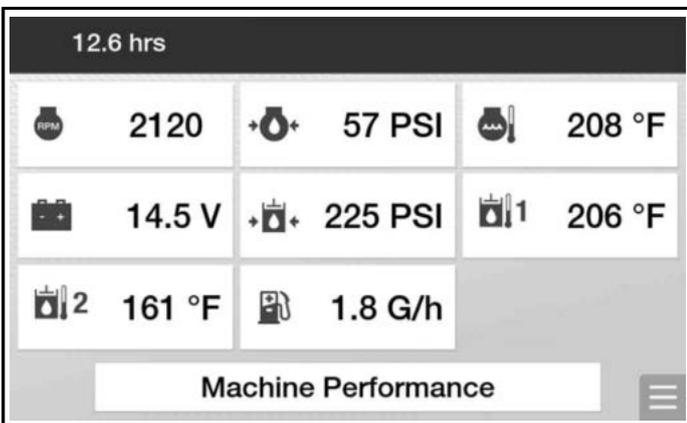
Frequently monitor the **GAUGES** [Figure 114] and **VITAL DETAIL** [Figure 115] screens for machine condition.
