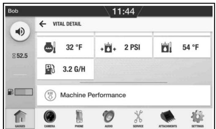
Frequently monitor the **GAUGES** [Figure 117] and **VITAL DETAIL** [Figure 118] screens for machine condition.
