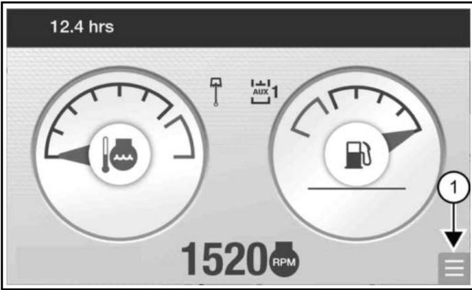
1. Select the navigation handle (Item 1) [Figure 400] to open the navigation bar.
