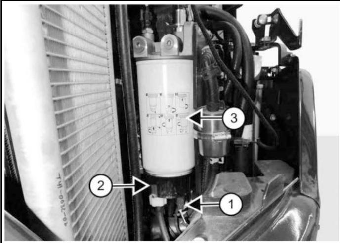
5. Disconnect the electric connector (Item 1) [Figure 344] from the bottom of the fuel filter.
