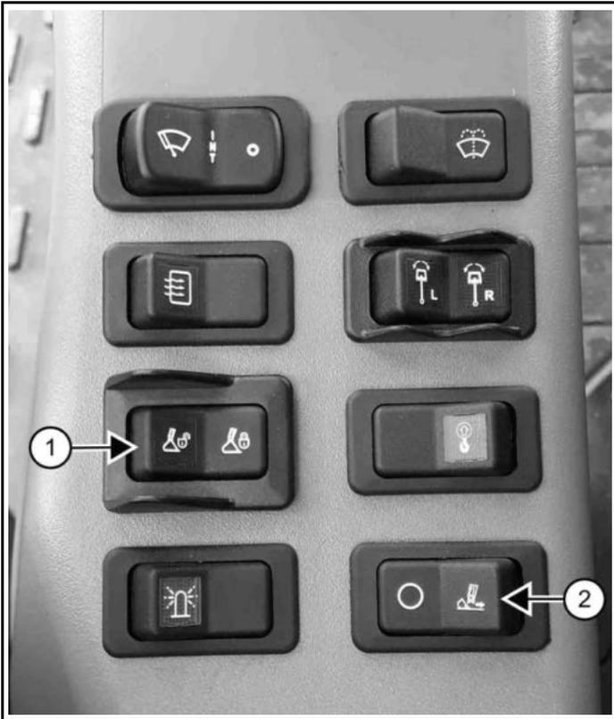
5. Press the coupler ON / OFF switch (Item 1) [Figure 175] to the left (ON) position to enable the quick coupler feature.
