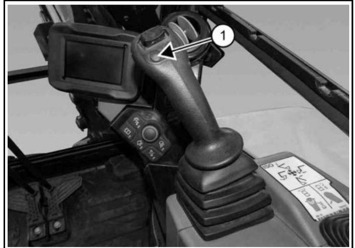
You can also press the right joystick button (Item 1) [Figure 20] to toggle between the camera and the current screen.
