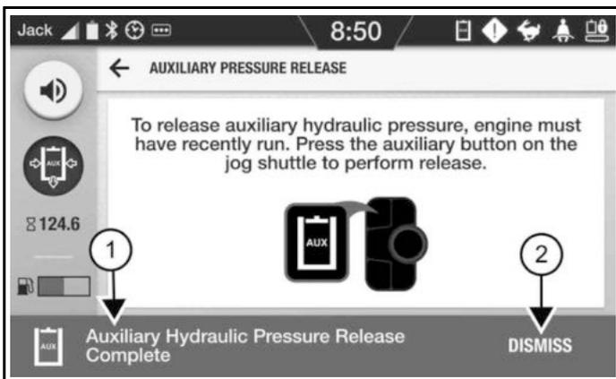
When the process is completed, a notification (Item 1) will appear indicating that the auxiliary pressure has been released. Press [DISMISS] (Item 2) [Figure 446].
