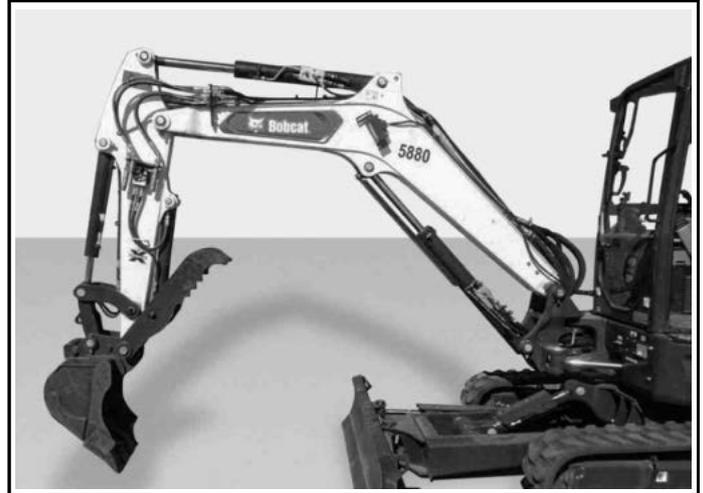
2. Place the bucket teeth on the ground with the teeth at the lowest point in the bucket movement arc [Figure 303].
