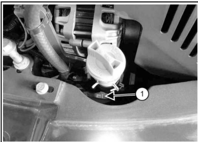
The engine serial number (Item 1) [Figure 2] is located on the side of the engine under the oil fill cap.
