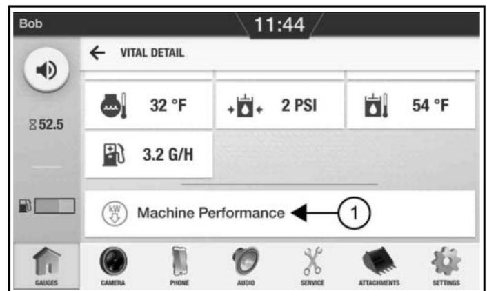
2. On the **VITAL DETAIL** screen, view a digital readout of the gauges. The screen provides real-time monitoring of:
