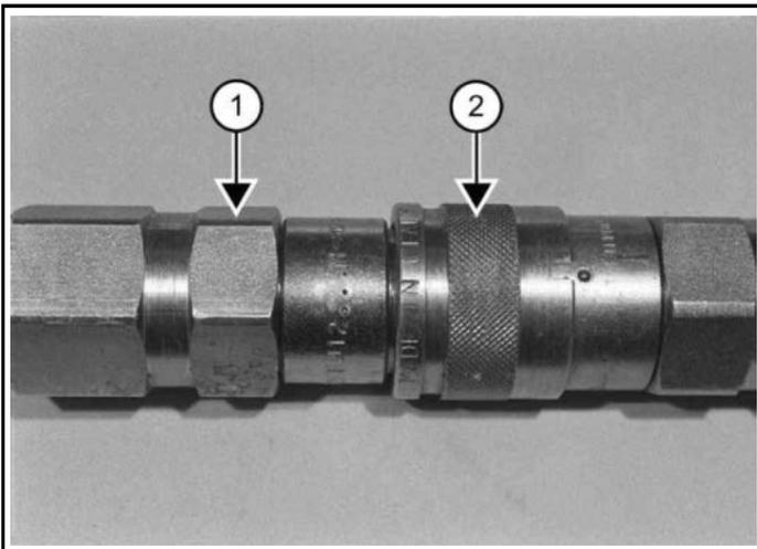
4. To disconnect, hold the male coupler (Item 1) and retract the sleeve (Item 2) on the female coupler until the couplers disconnect [Figure 56].
