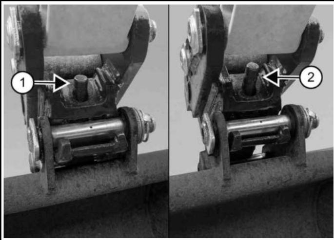
7. Visually inspect the indication bar to see if the coupler is fully engaged (Item 1) [Figure 166].
