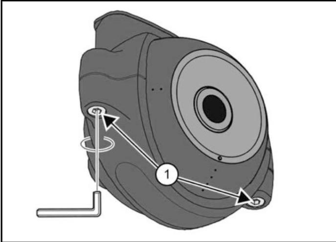
2. Loosen the screws (Item 1) [Figure 22] of the clamp holding the camera.
