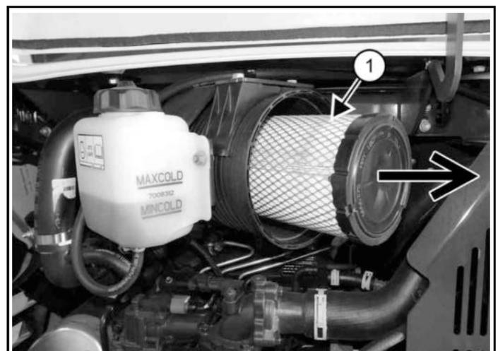
4. Pull the outer filter (Item 1) [Figure 337] from the air cleaner housing.
