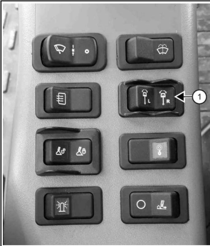
1. Push the Boom Swing switch (Item 1) [Figure 68] on the left console to the left to operate boom swing with the left joystick.
