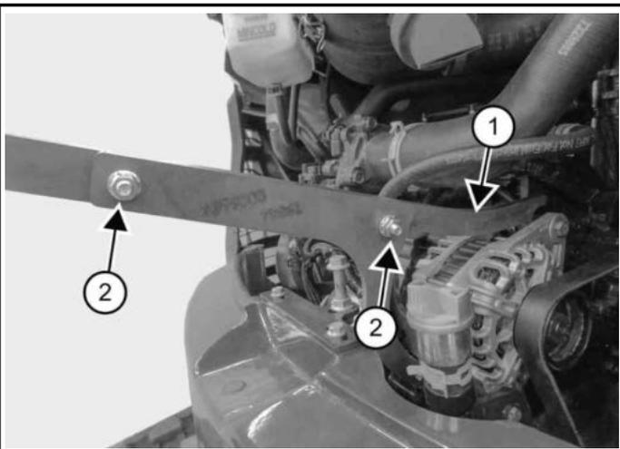
5. Position the upper alternator tool (Item 1) and install the bolts and nuts on the tool (Item 2) [Figure 385].
