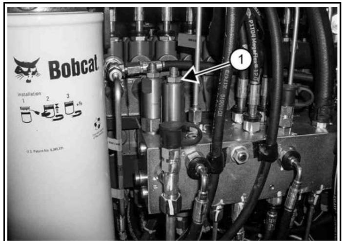
1. To decrease the track tension, loosen the nut shown here (Item 1) [Figure 379] on the pilot manifold and turn the hex head screw counterclockwise.
