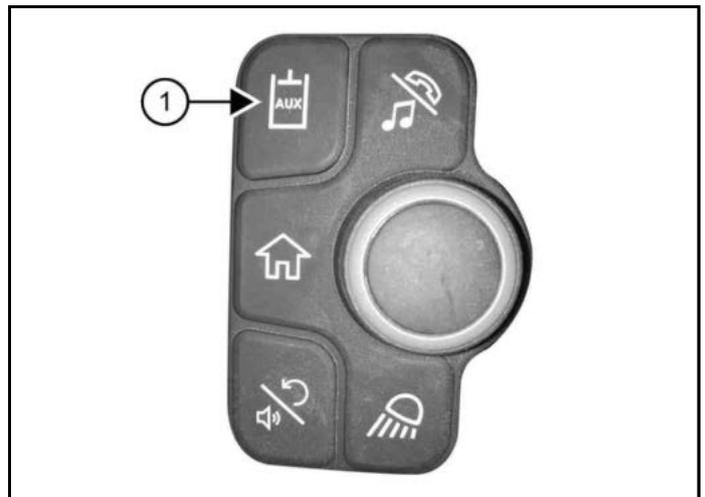
1. Press the AUX button (Item 1) [Figure 57] on the jog shuttle.
