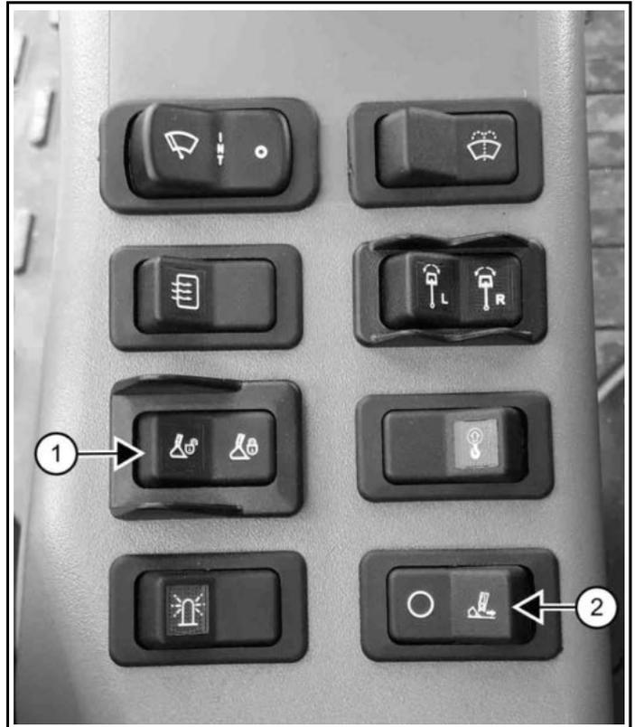
4. Press the coupler ON / OFF switch (Item 1) [Figure 183] to the left (ON) position to enable the quick coupler feature.
