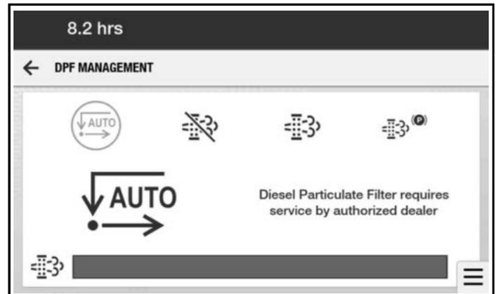
The machine will alert the operator when DPF service is required [Figure 372].
