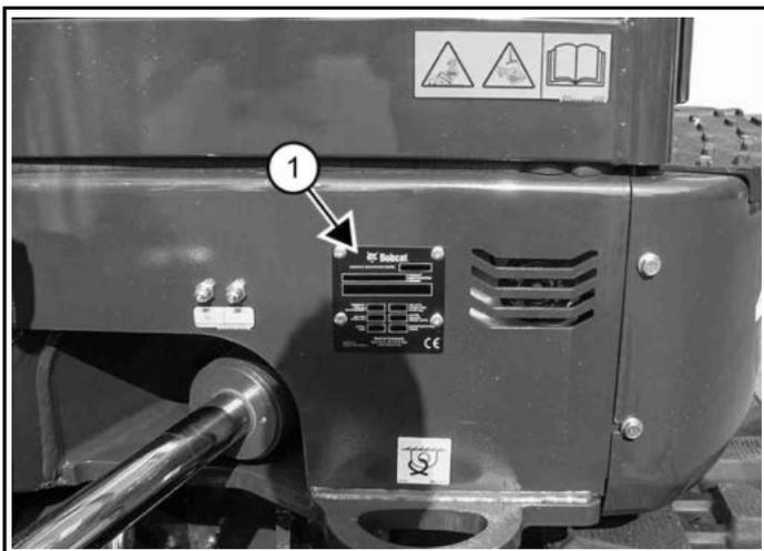
The machine serial number plate (Item 1) [Figure 1] is located on the frame of the machine in the location shown.
