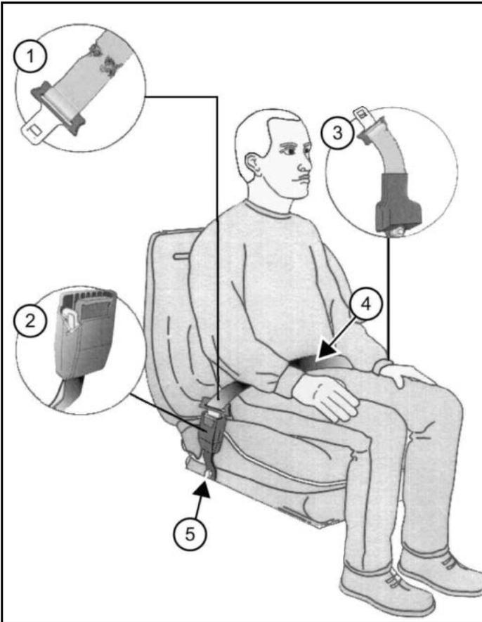
Check the seat belt daily for correct function. Inspect the seat belt system thoroughly at least once each year or more often if the machine is exposed to severe environmental conditions or applications.
