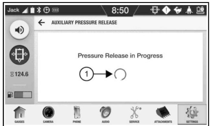
The spinner (Item 1) [Figure 445] will rotate until the Auxiliary Pressure Release procedure is complete.
