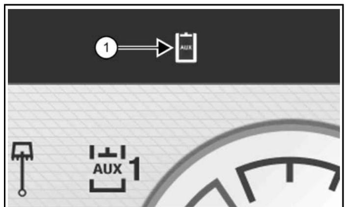
The auxiliary hydraulics icon (Item 1) [Figure 58] will turn ON.
