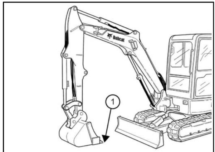
1. Set the bucket (Item 1) [Figure 243] on the ground surface where you are going to start the dig or on the surveyor mark to establish the starting ground position.
