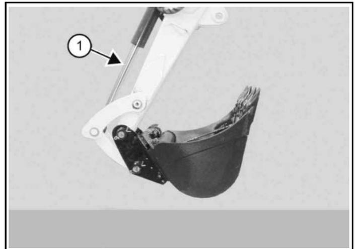
10. Extend the bucket cylinder (Item 1) [Figure 145] fully.
