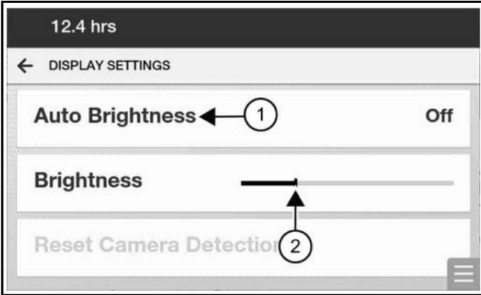
2. Select **[AUTO BRIGHTNESS]** (Item 1) [Figure 408] to turn it on / off. When on, the brightness will automatically adjust according to the ambient light.
