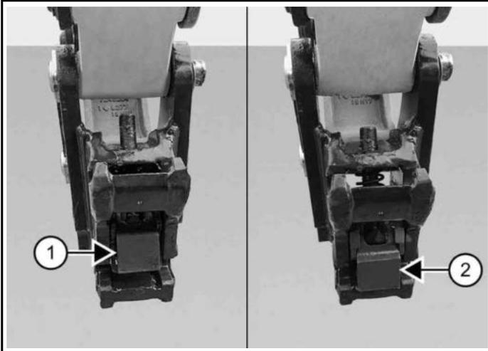
2. Inspect the quick coupler. If the wedge and the trigger are in the primed position (Item 1) [Figure 162], proceed to Step 4.
