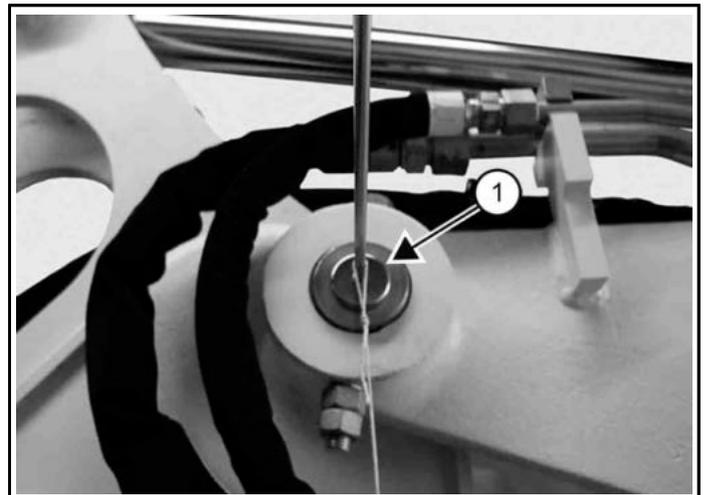
4. Install the magnetic tool on the arm pin (Item 1) [Figure 272].
