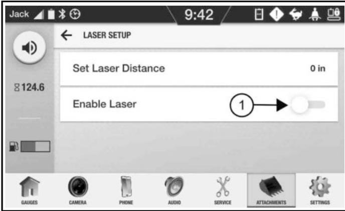
3. Enable the laser by moving the slider (Item 1) [Figure 298].
