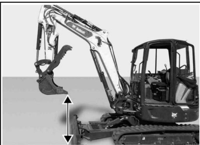
5. Measure how high the bucket teeth are off the ground [Figure 306].
