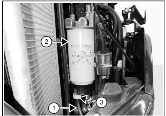
6. Locate the hose (Item 1) under the fuel filter (Item 2) and put a container underneath the upperstructure (hose should be routed down through the frame) [Figure 343].
