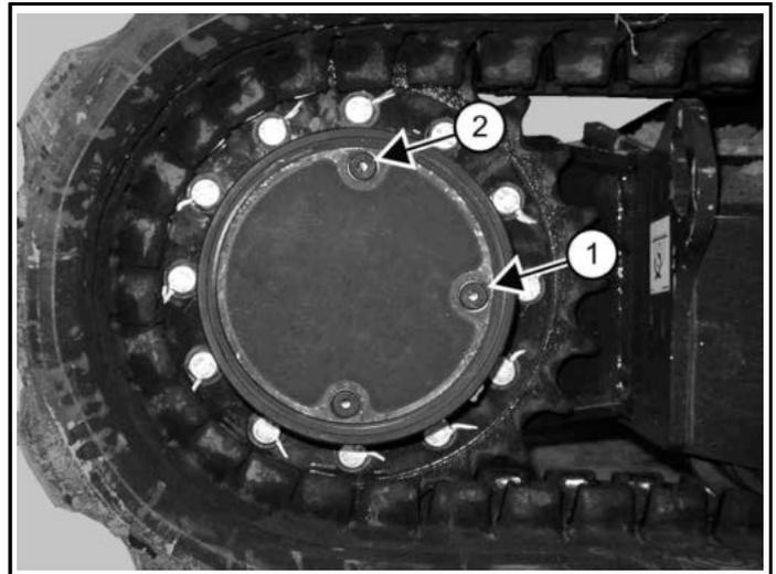
1. Park the excavator on a level surface with the plugs (Items 1 and 2) [Figure 381] positioned as shown.
