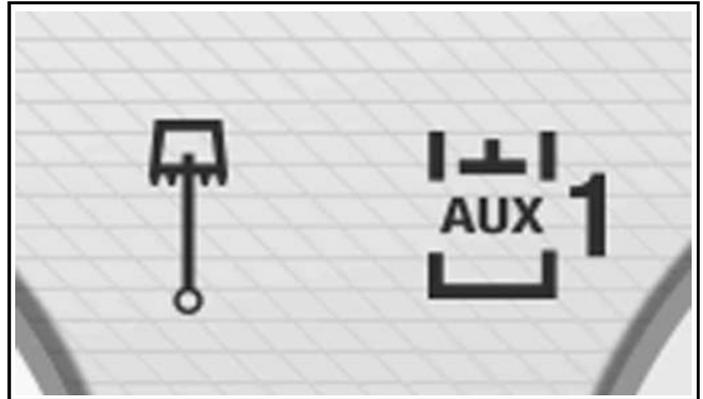
The display will indicate the left joystick controls boom swing and the right joystick controls primary auxiliary hydraulics [Figure 70].
