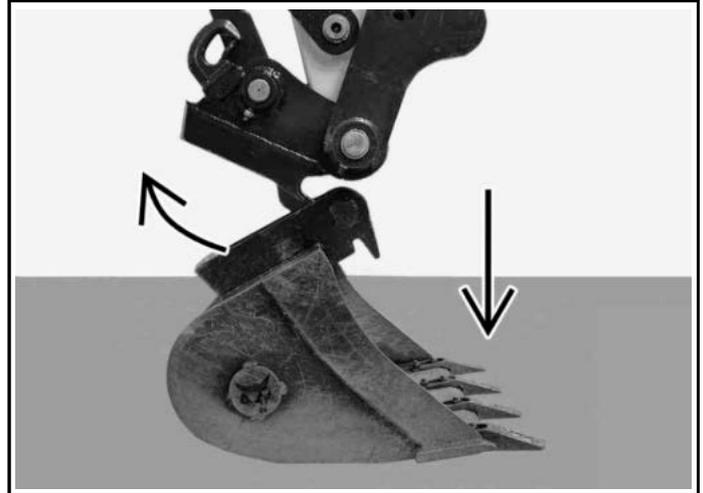
10. Move the arm away from the excavator until the quick coupler is clear of the attachment [Figure 185] or [Figure 186].
