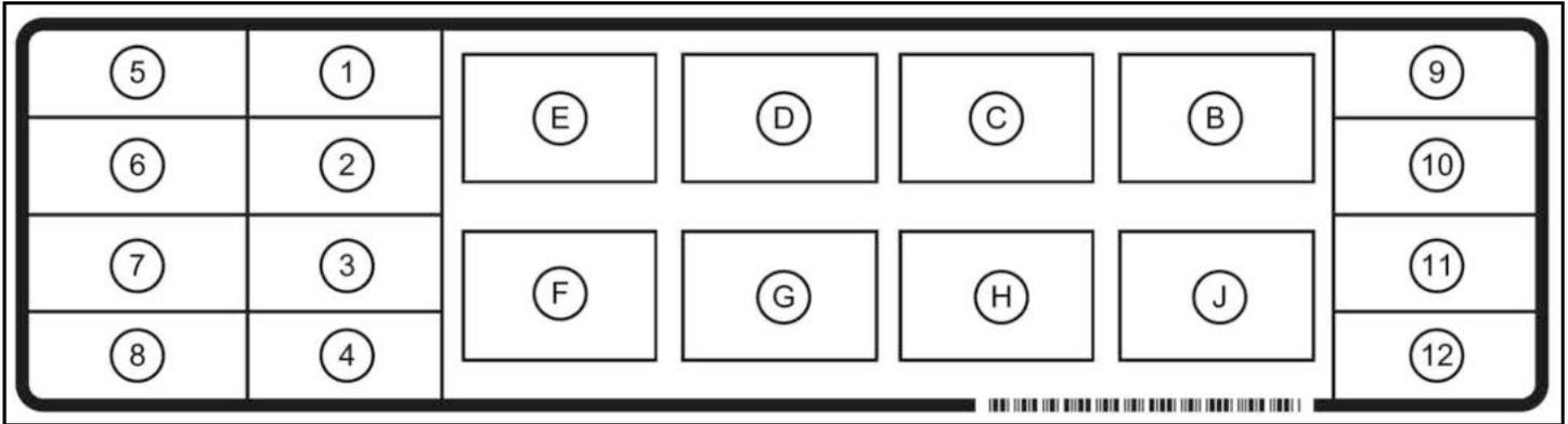
The location and sizes are shown in the table below and on the decal [Figure 358]. Always replace fuses using the same type and capacity. Relays are identified by the letter “R” in the Amp column.
