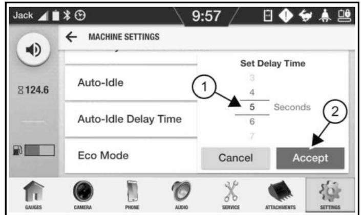
4. Swipe up or down (Item 1) [Figure 450] to select the auto-idle delay time to best suit the operating conditions.
