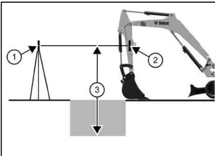
4. With the excavator arm vertical, raise or lower the boom and arm as needed until the laser (Item 1) strikes the receiver (Item 2) [Figure 299].
