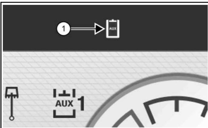
The auxiliary hydraulics icon (Item 1) [Figure 64] will turn ON.
