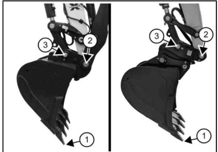
8. Measure the distance from the tip of the attachment (Item 1) to the centre of the inner pin (Item 2) [Figure 232] and enter this value.
