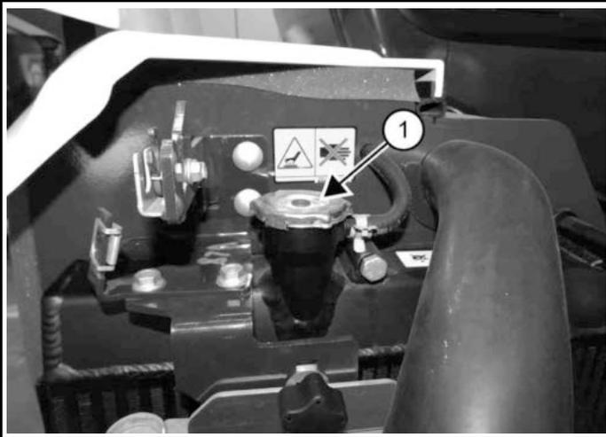
5. When the engine is cool, loosen and remove the radiator cap (Item 1) [Figure 354].
