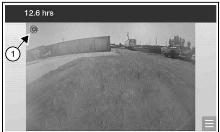
The rotating spinner icon (Item 1) [Figure 21] indicates you are viewing a live broadcast from the camera.
