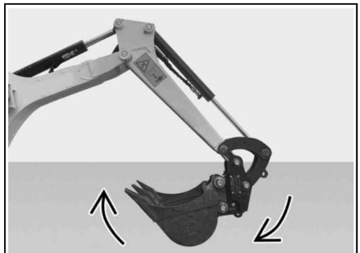
6. Extend the bucket cylinder and curl in the bucket [Figure 165] until you hear the wedge engage on the attachment back pin.
