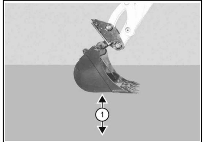
9. Raise the boom until there is approximately 500 mm (20.0 in) (Item 1) [Figure 144] of clearance between the bottom of the attachment and the ground.
