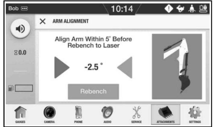
If the arm is not vertical when you try to rebench, the **ARM ALIGNMENT** screen [Figure 300] will remind you to align the arm vertically before rebenching. Adjust the arm and select **[REBENCH]**.
