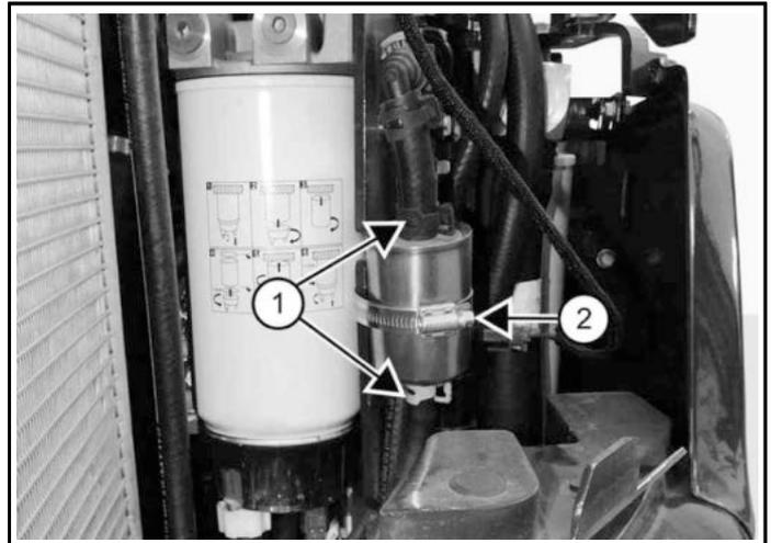
5. Pinch off the upper and lower hoses (Item 1) [Figure 345] to prevent spilled fuel while the hoses are disconnected from the pre-filter.
