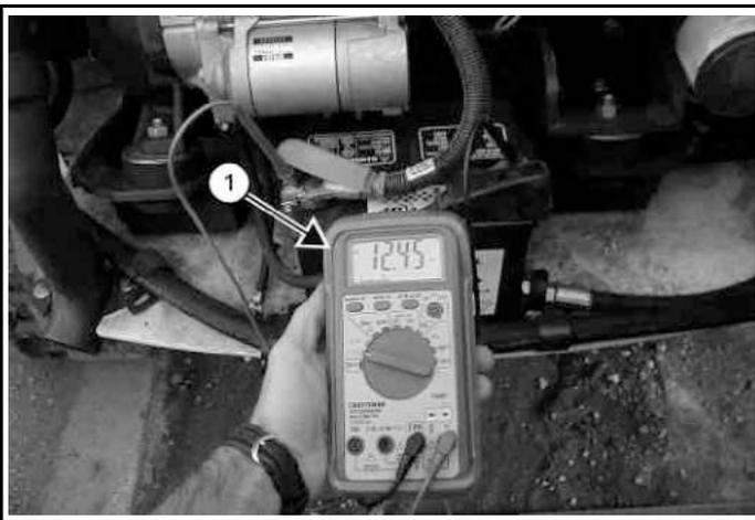
The simplest and most common check to determine battery state of charge is to use a digital multimeter or voltmeter (Item 1) [Figure 361].
