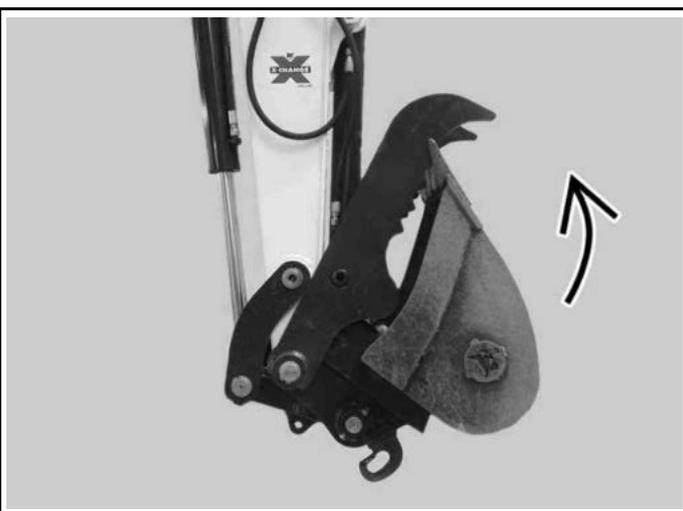
3. Move the right joystick (Item 1) [Figure 181] to the left (IN) to curl the coupler fully in toward the cab [Figure 182].
