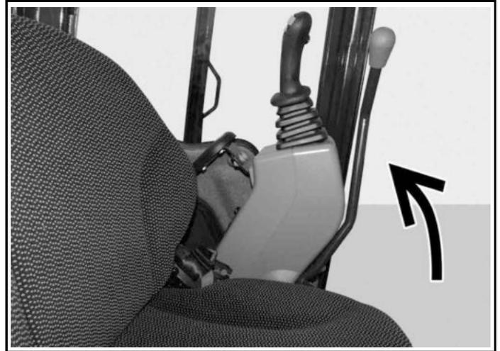
When the left console is raised [Figure 318], the hydraulic joysticks and traction system must not function.
