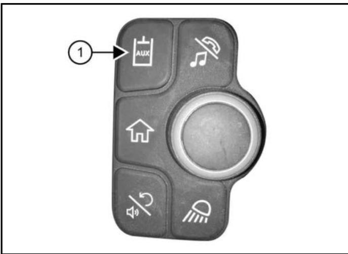
1. Press the AUX button (Item 1) [Figure 63] on the jog shuttle to activate auxiliary hydraulics.
