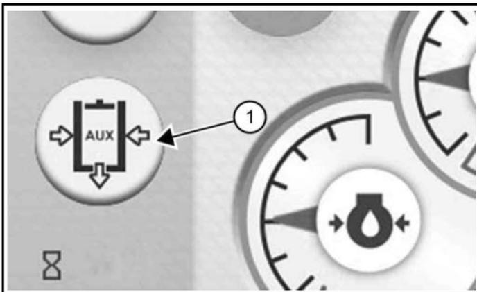
The Auxiliary Pressure Release icon (Item 1) [Figure 443] will be visible when releasing auxiliary pressure is possible.
