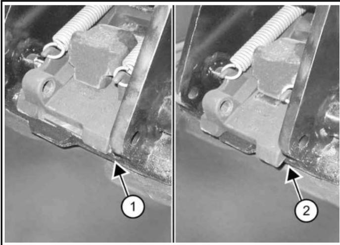
Visually inspect the quick coupler latch to the bucket mount [Figure 149]. The latch must be fully engaged (Item 1) [Figure 149].
