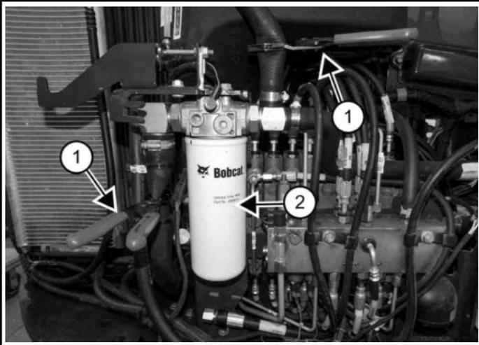
5. Install locking hose pliers (Item 1) [Figure 367] on the hoses running to the filter housing.
